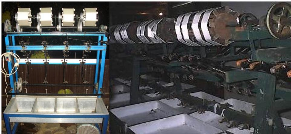
Gambar 63. Mesin Reeling semi otomatis
